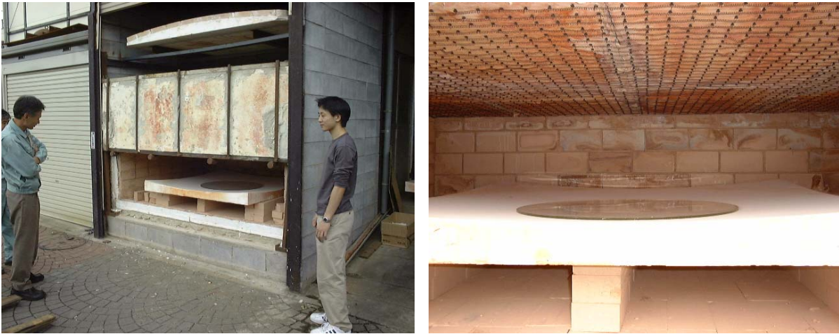
FIG. 2.6: Electric oven (left) and ceramic mold (right) used for the production of segment mirror.
