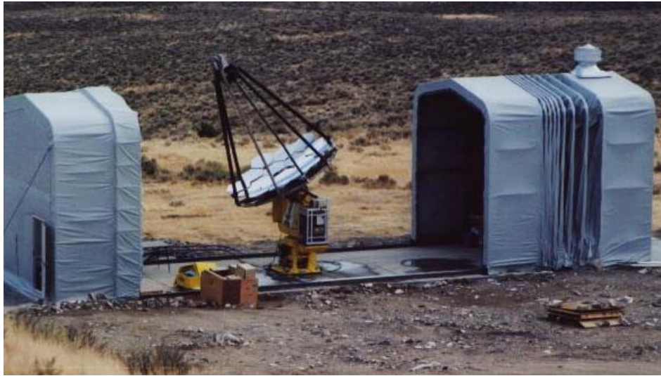
FIG. 3.17: Optical receiver for atmospheric monitoring in Telescope Array experiment. The mirror of 3m diameter is mounted on the alt-azimuth. The pointing resolution is 1/1000 degree and the maximum rotating speed is 5 degree/sec.
