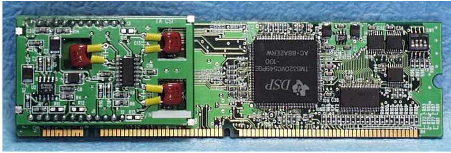
FIG. 2.26: Prototype signal finder sub-board for one channel.
