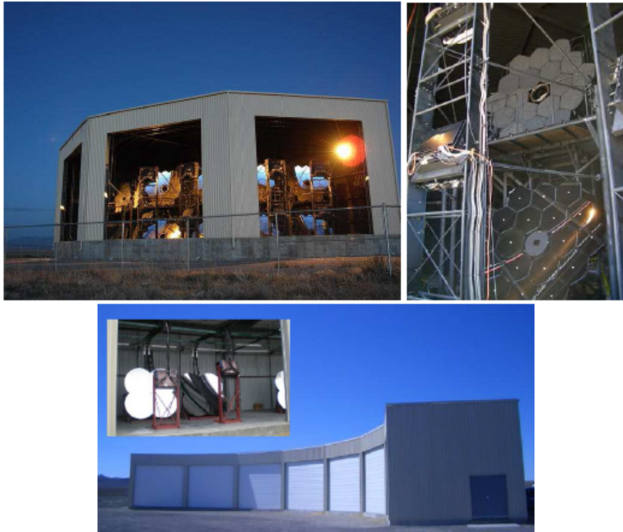
Figure 2.4: The FD stations of the TA experiment [35]. The upper photograph shows the BRM station and a pair of FD telescopes designed to cover lower and upper elevations of the sky. The lower photograph shows the MD station and a pair of FD telescopes covering the sky's lower and upper elevations. Showing the BRM station and the MD station have different instruments.
