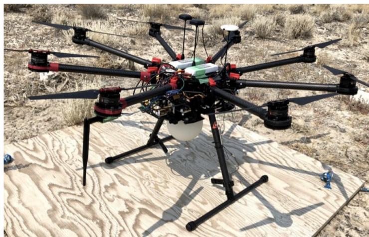
Figure 2.13: The multirotor module Opt-copter developed for calibrating FDs of the TA experiment [41].
