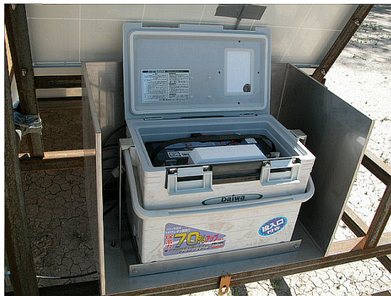
Fig. 14: The stainless-steel box at the backward of the solar panel. Battery is set in the cooler box to keep moderate temperature (left figure). The cooler box and electronics for the data acquisition are set in the stainless-steel box for the protection from the rain and wind (right figure). This stainless-steel box is closed and locked after deploying.
