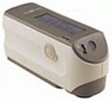
Fig. 24: The spectrophotometer for measurement of the mirror reflectance (KONICA MINOLTA CM-2500d).
