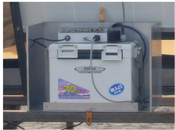
Fig. 14: The stainless-steel box at the backward of the solar panel. Battery is set in the cooler box to keep moderate temperature (left figure). The cooler box and electronics for the data acquisition are set in the stainless-steel box for the protection from the rain and wind (right figure). This stainless-steel box is closed and locked after deploying.
