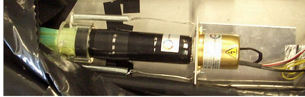
Fig. 13: The PMT for SD (Electron Tube 9124SA) with 9/8-inch diameter. It is covered with Mu-metal for protection from geomagnetism.
