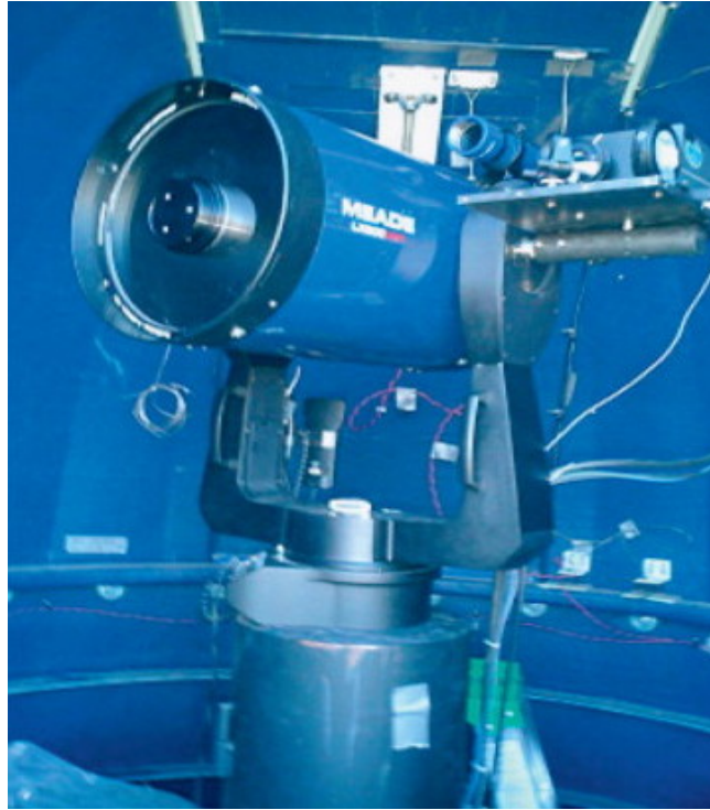
FIGURE 2.31: A picture is LIDAR's optical system (telescope, laser, etc).
