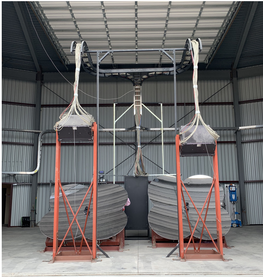
FIGURE 2.8: Photo of the TALE telescopes. Left one is ring 4 telescope (#17), and right one is ring 3 telescope (#18). Each telescope has the clover-shaped spherical mirror, the black box shaped PMT camera, which supported by orange stands and connected to the electronics crate located at center of both mirrors.
