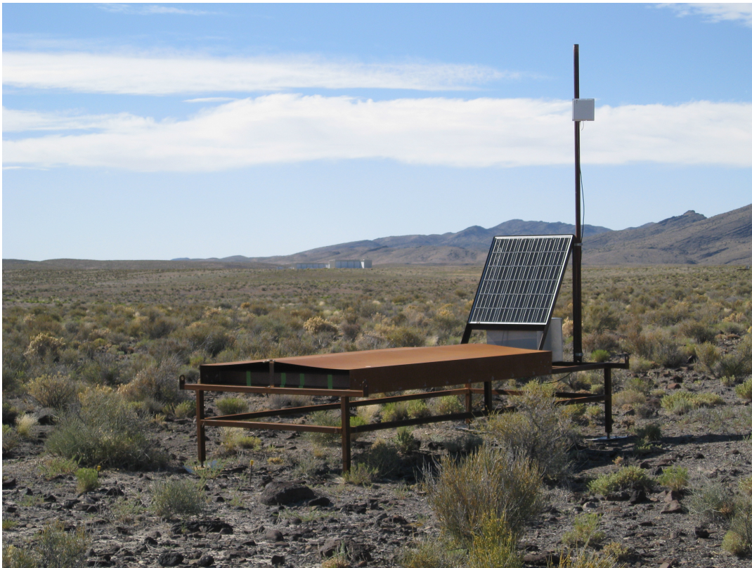
FIGURE 2.21: Photo of the TALE Surface Detector. The TA MD / TALE buildings are seen far from this SD.
