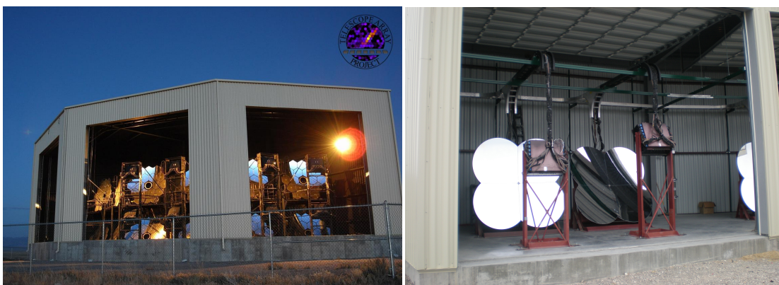
FIGURE 2.2: Left: A photo of Black Rock Mesa fluorescence station. These are three bays, each with four telescopes. The Long Ridge fluorescence station is same structure as BRM station. Right: A photo of Middle Drum fluorescence telescopes.
